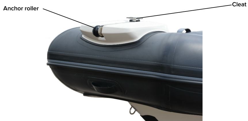
Fig. 33. Bow step plate.
