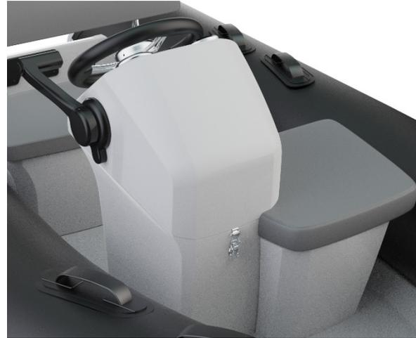
Fig. 28. Additional console seat for S300L, S330L.
