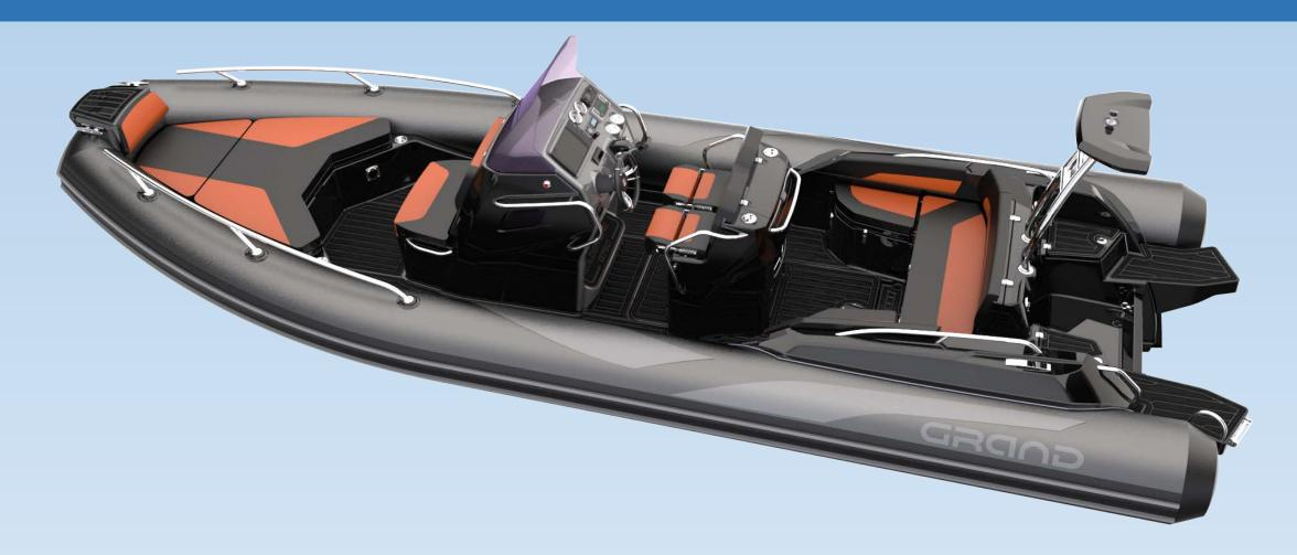
The G750 model completes GRAND's Golden Line Cruiser range fitting neatly between the G650 and G850 models. It offers the optimum balance between a high-performance larger RIB and a sumptuously appointed contemporary family boat. GRAND's proven High Step Deep-V Hull design ensures excellent maneuverability combined with dynamic stability and impressive speed capability.
