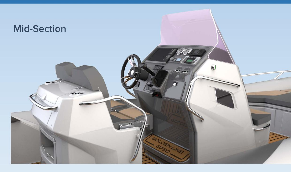
The newly designed steering console is centrally positioned for optimal balance, drivability and sea keeping performance. Two stainless steel safety handrails are installed on each side of the console to support the driver and the passenger.
