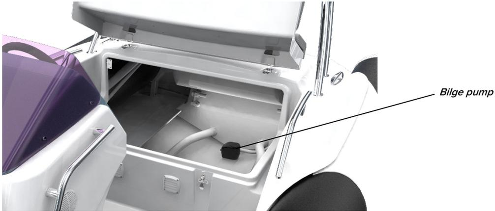
Fig. 23. Interior space of rear compartment with bilge pump inside of additional section.
