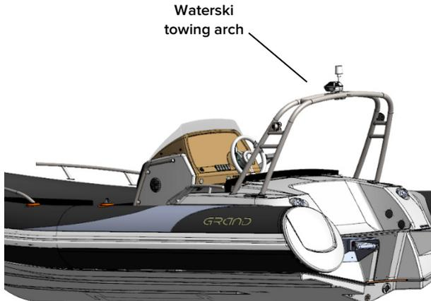
Fig. 41. Waterski towing arch.
