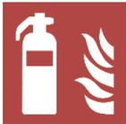
Fig.4. Symbol of designated place of portable fire extinguisher.
