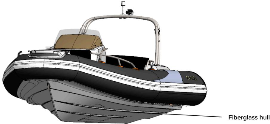
Fig. 42. Fiberglass hull.
