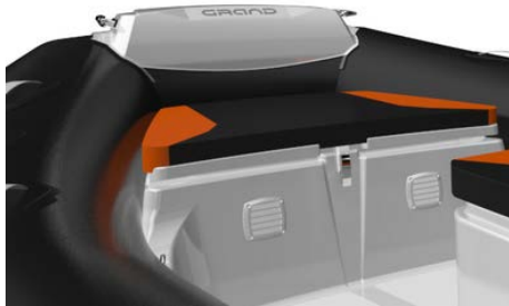
Fig. 1. Ventilation openings on the bow locker.
