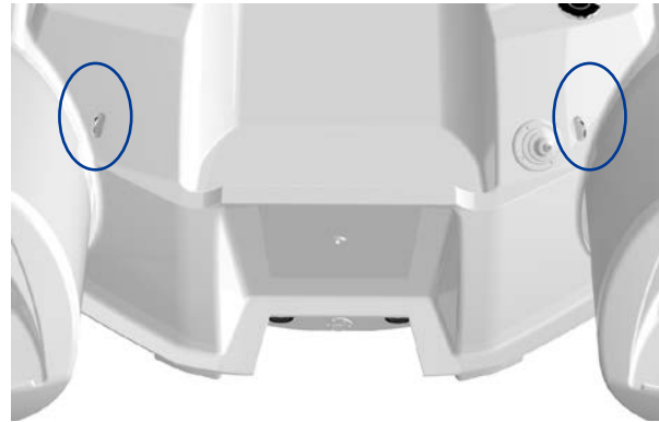
Fig. 25. Rear lifting eyes, 2 positions.
