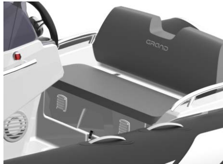
Fig. 2. Ventilation openings on the rear dry storage compartment.
