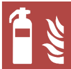
Fig.4. Symbol of designated place of portable fire extinguisher.
