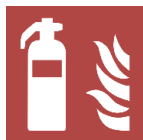
Fig. 8. Symbol of designated place of portable fire extinguisher.
